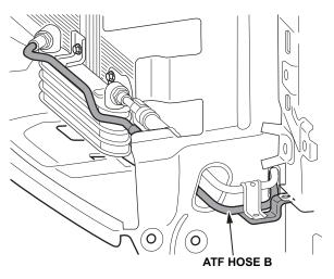
14. Install the hose bracket using a 6 x 16 mm washer bolt.
