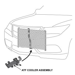
9. Install the ATF cooler with three 6 x 20 mm washer bolts.
