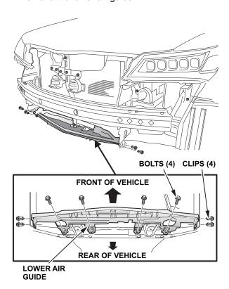
5. Remove the front bumper center lower grille NOTE: If equipped, remove the parking sensor sub harness clamps.
