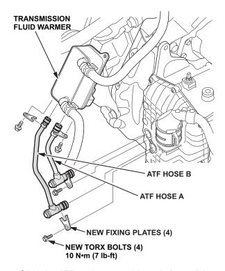
8. Slide the ATF cooler assembly up in front of the radiator as shown.
