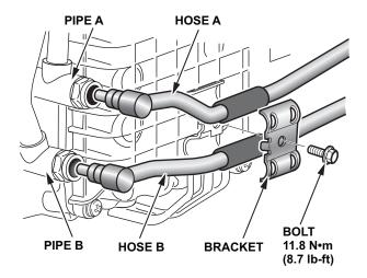
17. Secure the hoses with the bracket using one 6 x 16 mm washer bolt as shown.
