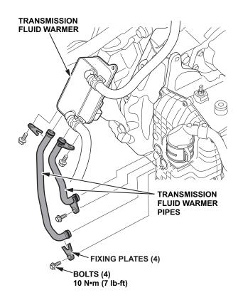
7. Make sure the connection points are clean and free of debris, then install ATF pipe A and ATF pipe B using the new fixing plates and Torx bolts supplied in this kit.
